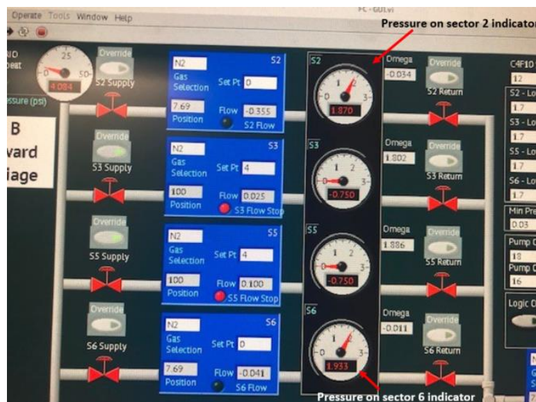
Screenshot of LTCC gas system pressure controls GUI
